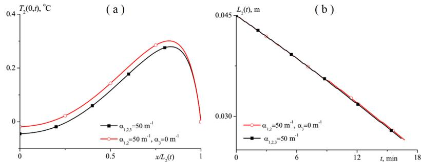
Figure 4: The temperature field in the ice layer at the end of melting (a) and the melting rate (b) of the ice layer, depending on the  $\alpha_{gas,j}$ .
