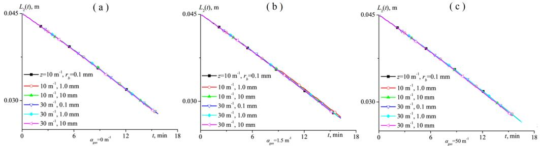
Figure 3: Dynamics of melting of the cloudy ice layer at different values of the anisotropic scattering parameters and  $\alpha_{gas}$  (See nomenclature in Fig. 2).
