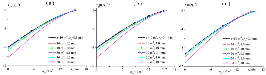
Figure 2: Dynamics of temperature growth of the left non-irradiated boundary of the ice layer in the melting stage at different values of the scattering parameters and  $\alpha_{gas}$  ( $a$  is the  $\alpha_{gas} = 0$ ,  $b$  is the  $\alpha_{gas} = 1.5m^{-1}$ ,  $c$  is the  $\alpha_{gas} = 50m^{-1}$ ).
